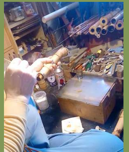
Above: Miura Ryūho in his Tokyo studio, April 2017: shakuhachi parts, RM handle tools, urushi , and tools, tools... (top right: applying ji paste to the inside of the bamboo; bottom right: brushing the first layer of ki ( seshime ) urushi onto the joint tenon .)
