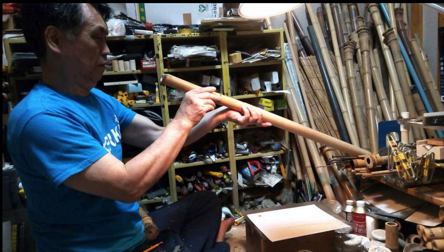
Miura Ryuho in his Akita studio using the ‘center tool’ to check the nakatsugi cut. Summer 2019 (Photo: Thorsten Knaub)
